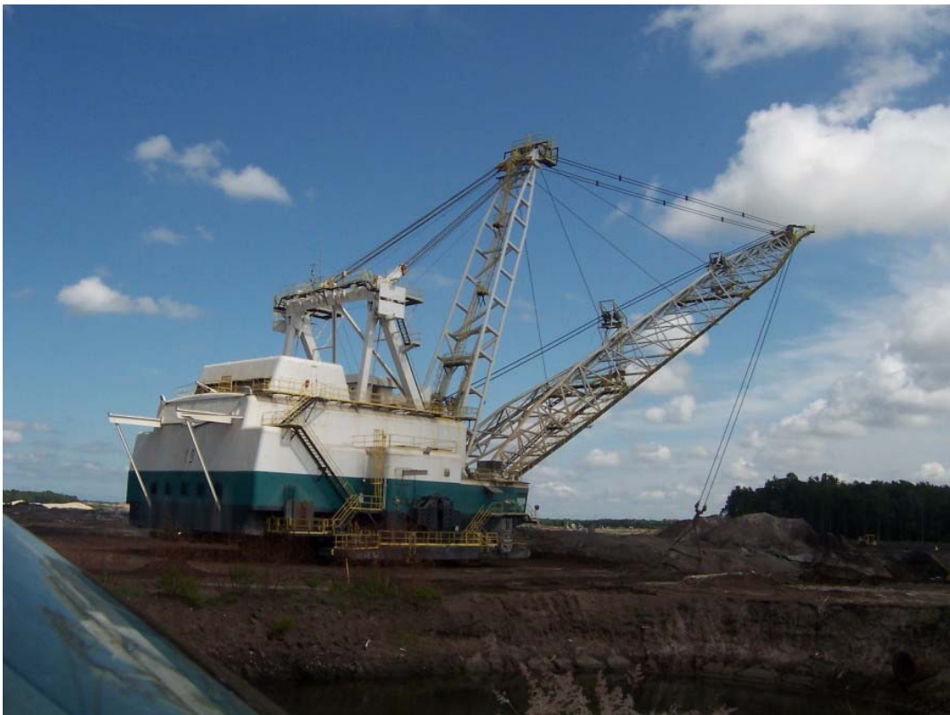
Dragline mining for phosphate at the Four Corners Lonesome Mine (Credit Florida Department of Environmental Protection)
